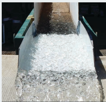
Figure 1: Clear water with no detached sediment was observed at shear stress of 32.7 pa and at a flow rate of 1290 L/min.
