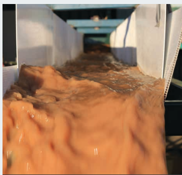
Figure 2: Control surface showed very high levels of suspended solids at shear stress of 15 pa and at a flow rate of 900 L/min.
